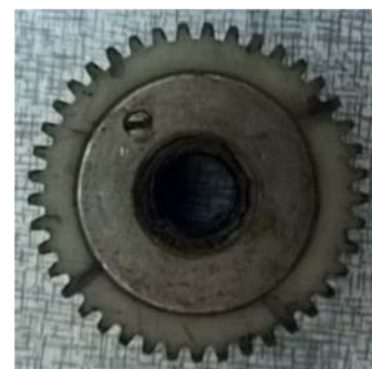
Figure 19. Shaft and bushing in 41T Gear.
