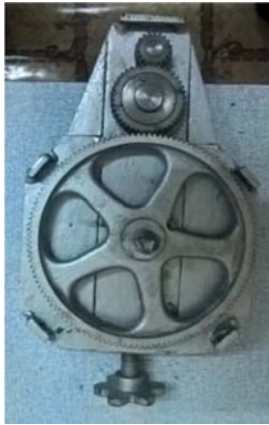
Figure 21. Assemblage of three gear train.
