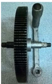
Figure 17. Shaft secured on gear 137T.
