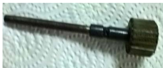
Figure 20. Spindle imbedded into 19T gear.
