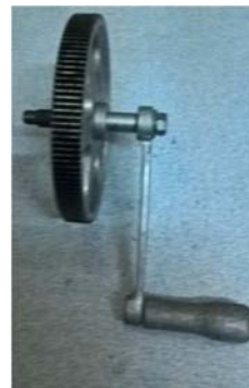
Figure 18. Handle fitted to the shaft.
