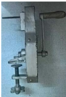
Figure 23. Handle Fitted onto shaft.
